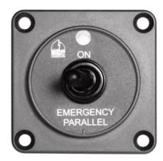
Remote emergency parallel VSS control is achieved by using a remotely mounted momentary switch, such as the BEP #80-724-0007-00 unit (pictured at right), which also features an LED to show the VSS status. When operated, the remote switch engages the 720-MDVSO contacts, paralleling the batteries, for a 10 minute period, for example to get an engine started following a flat start battery.
